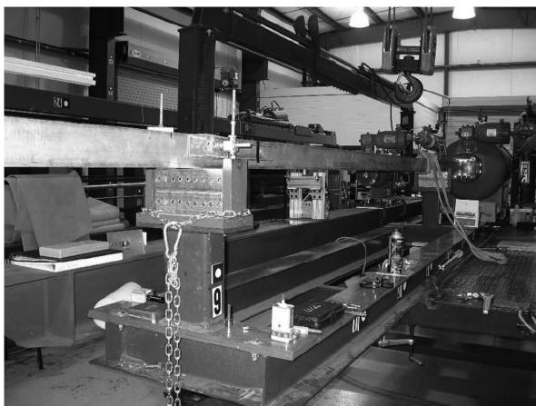
Fig. 2 Compressed gas gun, steel disk projectile with sabot, and aluminum cylinder projectile with sabot.
